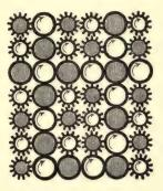
FIG. 45.—Section of a uniform magnetic field with two rails and a slider in it. It the slider be moved to or fro, the wheels inside get initially compressed or extended, and thereby gain or lose energy respectively, thus exciting the state of slip known as induced current.
